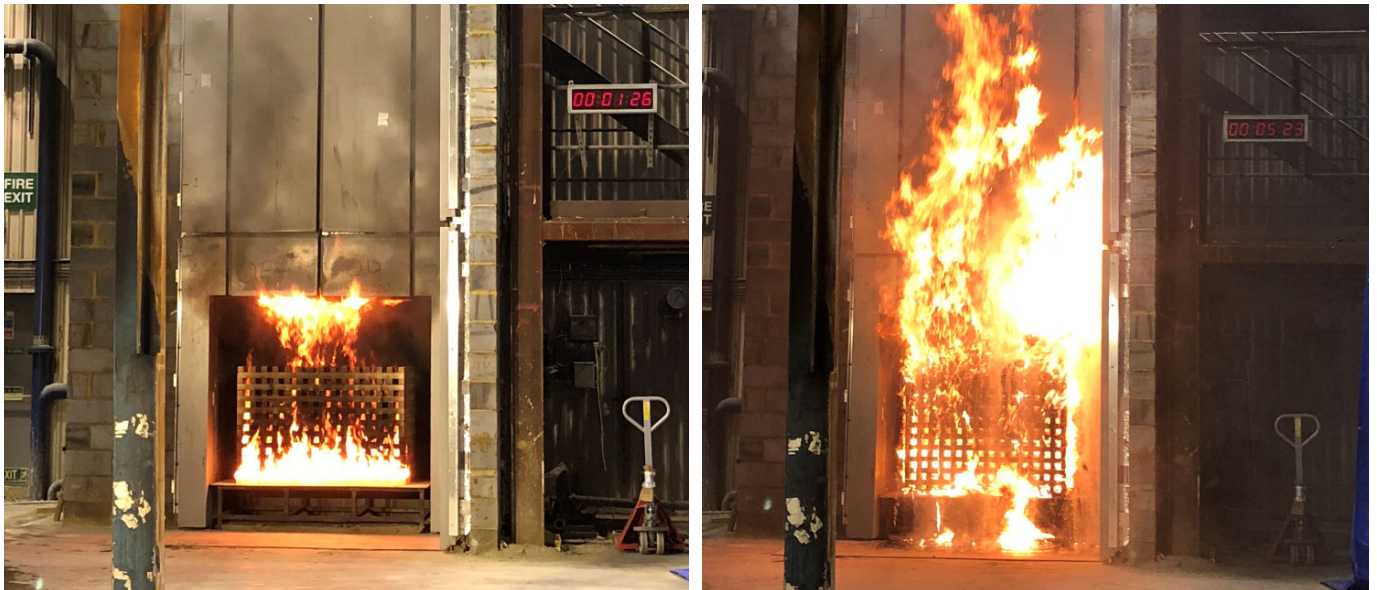
Figure 5.9: photographs of a BS 8414 test in operation
