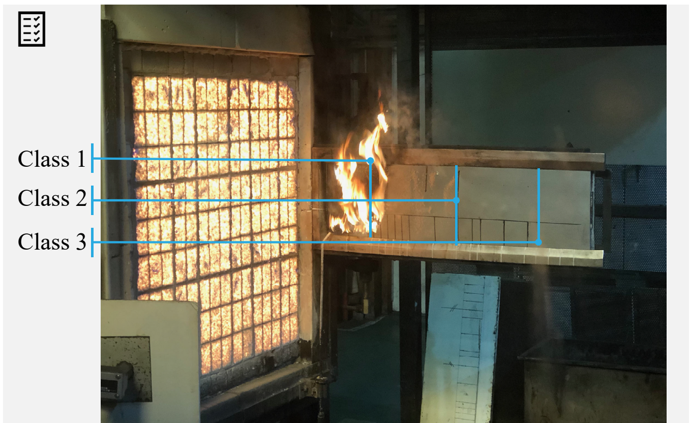
Figure 5.2: Image of BS 476-7 test in operation
