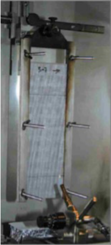
Figure 5.5: Picture of sample about to undergo ISO 11925-2 test
